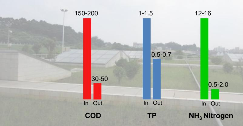
5 hours HRT in each tank – 3 tanks in series - Each tank is 10m<sup>3</sup>
